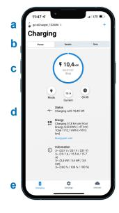
The "Charging" tab of the go-eCharger app gives you direct access to the most important functions for starting, stopping and monitoring charging processes.
