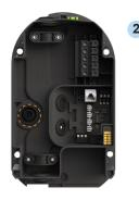
For rear cable routing it is recommended to fit the supply cable through the rear Wall Mount hole **before** alignment and marking the screw holes.
