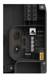
Pop out the small rubber grommet at the selected cable entry point: top or bottom.
