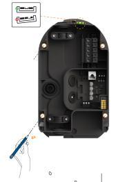
Use the built in spirit level and center markings for alignment.
