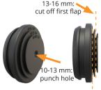
16-20 mm: cut off second flap Cut (with box cutter) or punch (e.g. with a pen) the grommet at the indicated position to create a hole at the required cable diameter. **Recommended cutting options are shown on the left.**
