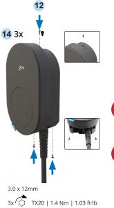
Secure the Charger in place using 3x TX20, length 12 mm screws and a Torx screwdriver, applying a torque of 1.4Nm ± 0.1Nm.
